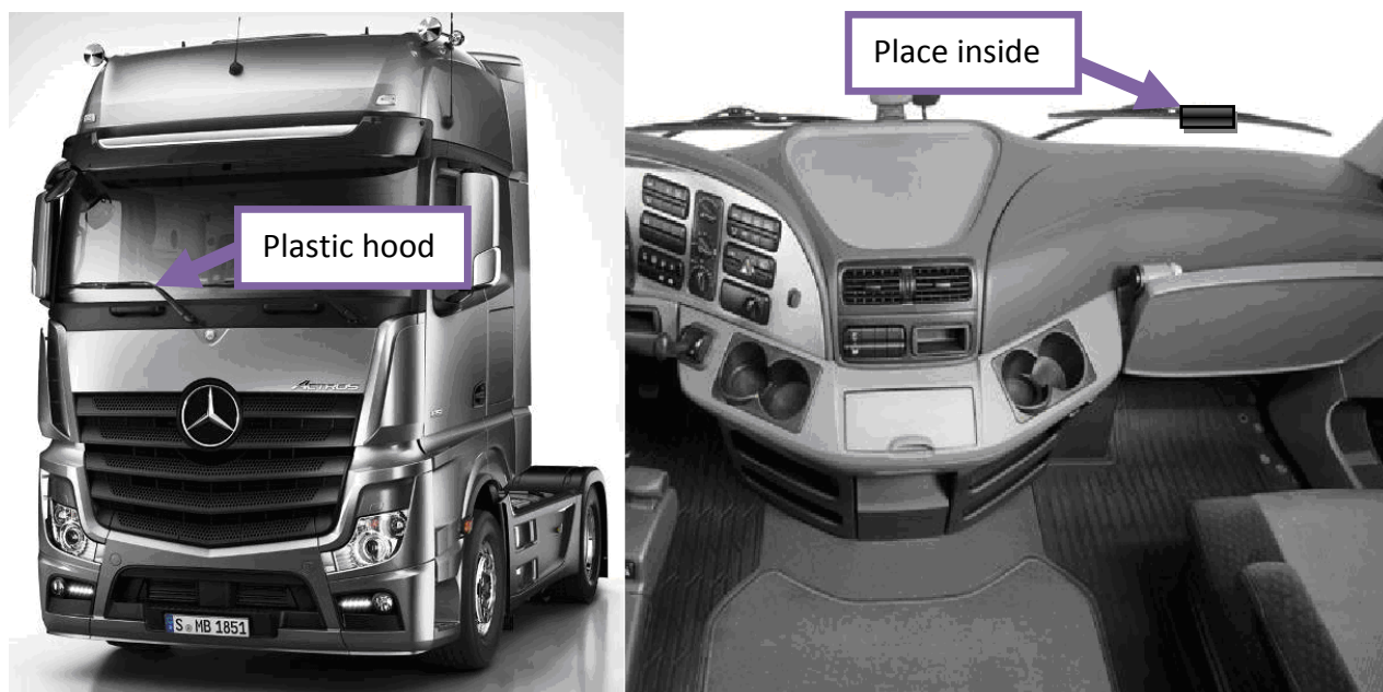
Figure 58. Possible mounting places in trucks
