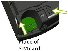
Insertin g SIM card position NOTE: If the red GSM LED is blinking check if the SIM card is placed correctly, or the PIN code is removed.
