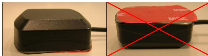
Figure 75 Correct GNSS antenna mounting
