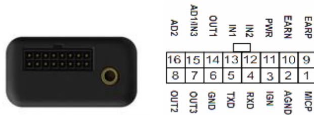
Figure 2. The 16 PIN connector on the GV320
