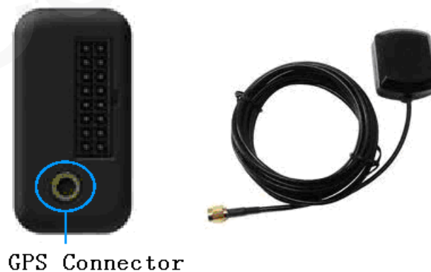
Figure 8. GPS Antenna of GV320
