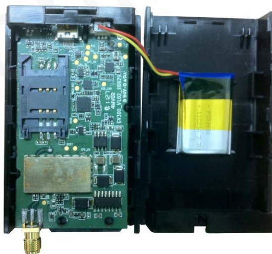
Figure 6. Backup Battery Installation
