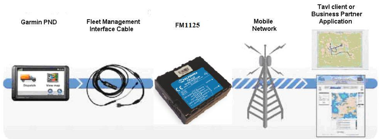
Figure 63 FM1125+Garmin operational scheme
