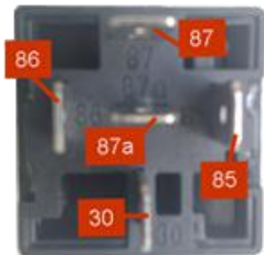
Bottom of relay Wiring Diagram
